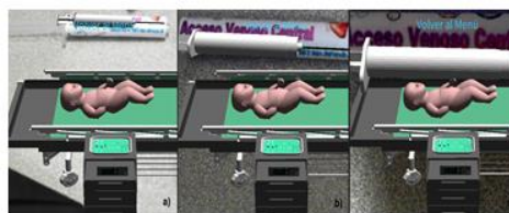
Fig. 6. Tracking quality using Microsoft Lifecam Studio webcam with a) halogen lights on, b) shadow over the camera, c) lights off
