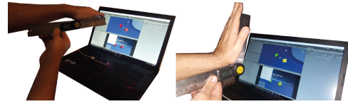
Fig. 5. Orientation validation with a ruler in 0 degrees and 70 degrees extended.
