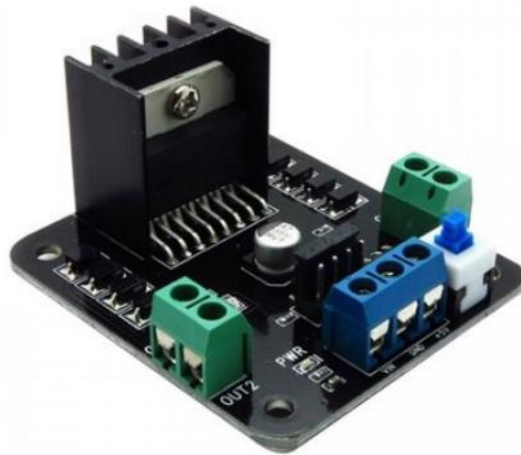
Figura 4.45. Driver puente H
