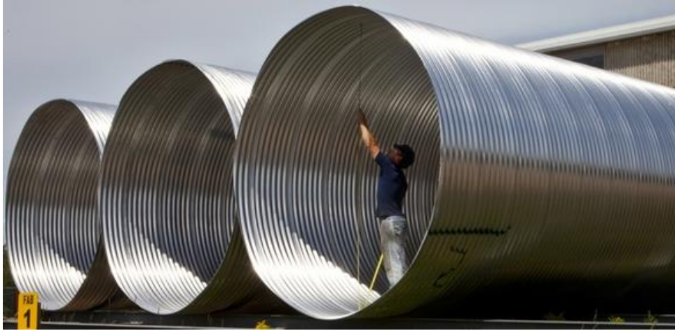
Ilustración 7 Inspecting corrugated steel pipe for sale. www.aill.ca
